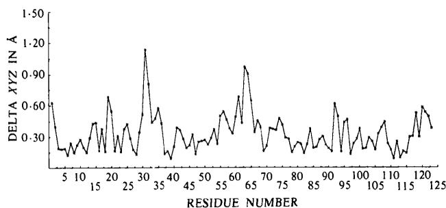
Fig. 3. Average deviations for the N, C<sup>α</sup> and C atoms after optimal superposition of the atomic positions of phospholipase A<sub>2</sub> (Dijkstra *et al.*, 1981) and prophospholipase A<sub>2</sub> after refinement A (Table 1).
